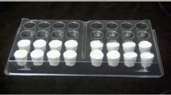
Figure 1. High impact polystyrene tray with 16 filter paper lined, pesticide treated cells into which one N. cucumeris was transferred and sealed.
