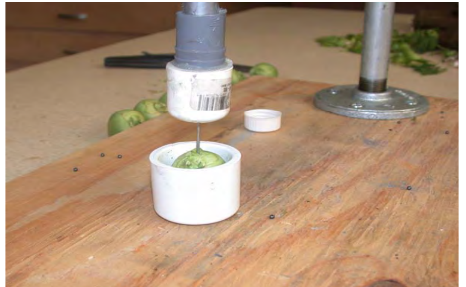
Measuring carpel wall toughness using a penetrometer
