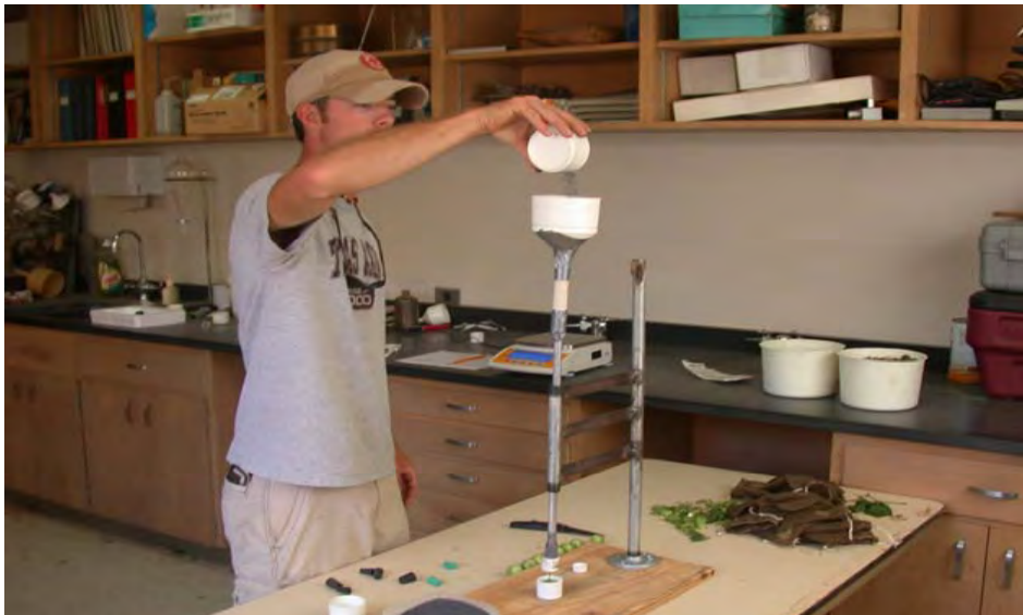
Measuring carpel wall toughness using a penetrometer
