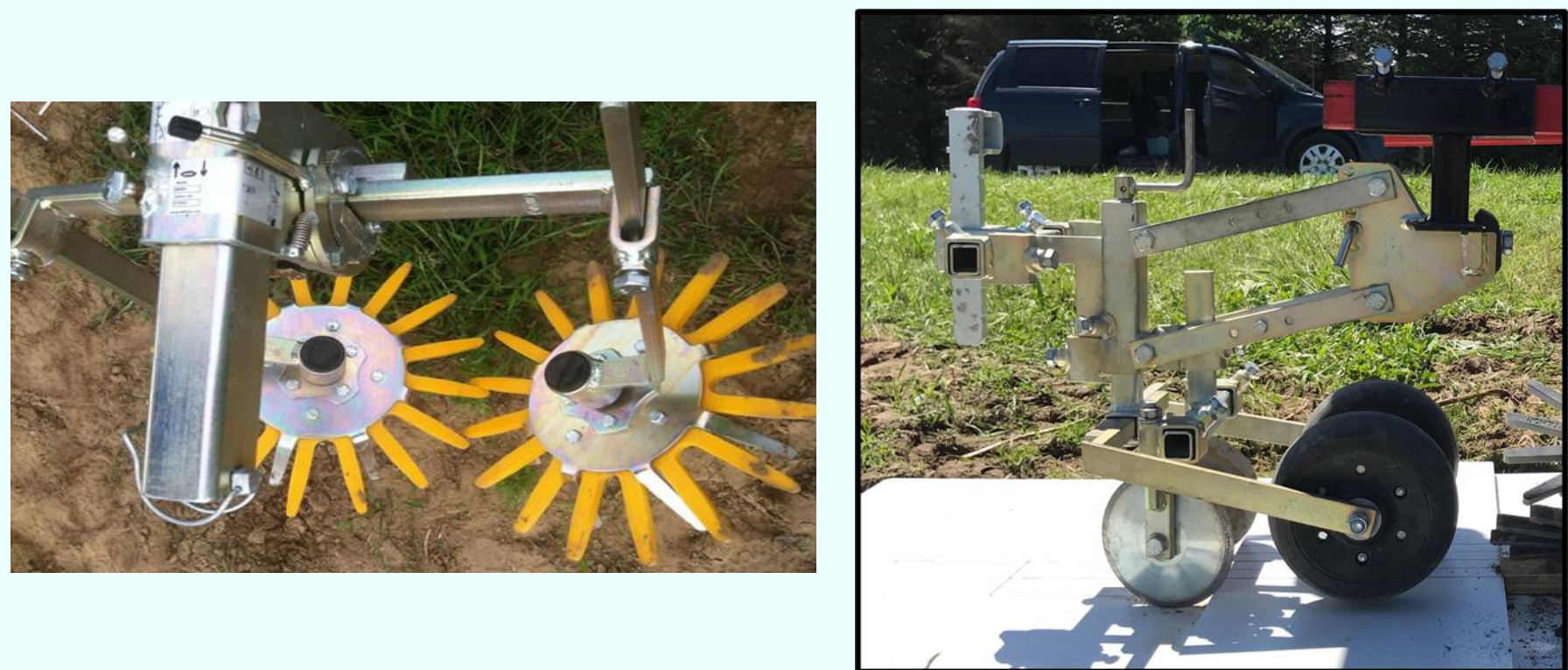
Fig. 2: Mechanical Cultivation tools a. Finger weeder primarily uproots weeds b. Hilling Disk primarily buries weeds
