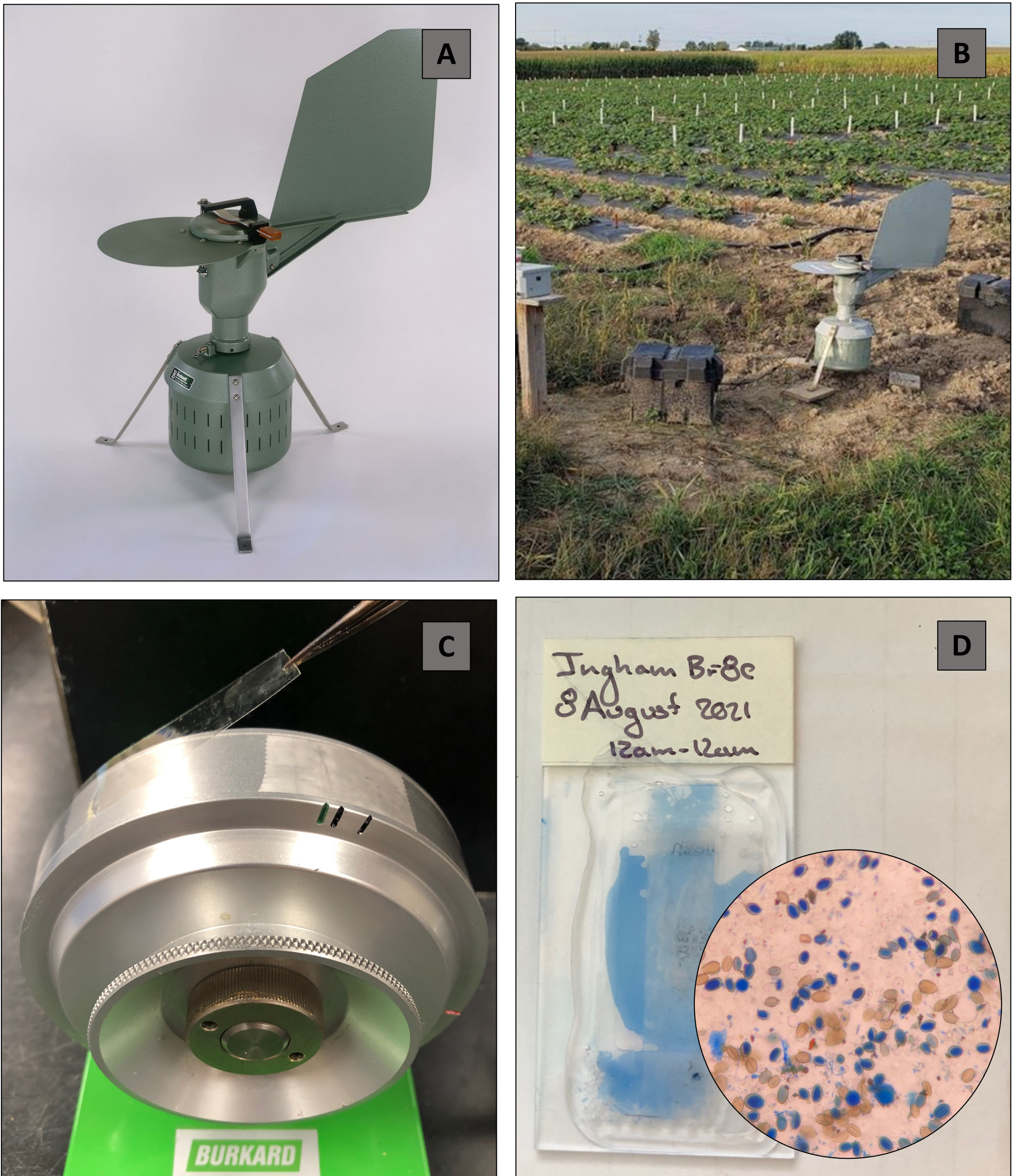
Figure 2: Components of spore trapping (A) Burkard volumetric spore trap Photo credit: http://burkard.co.uk/product/7-day-recording-volumetric-spore-trap (B) Spore trap in field (C) Spore trapping reel (D) Spore trap tape mounted on slide and sporangia visible on slide at 200x magnification under light microscope.
