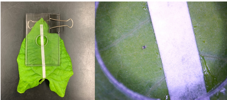
Setup for Tetranychus urticae behavioural assays, where half of the bean plant leaf is treated with a compound of interest, and half of the leaf is untreated.
