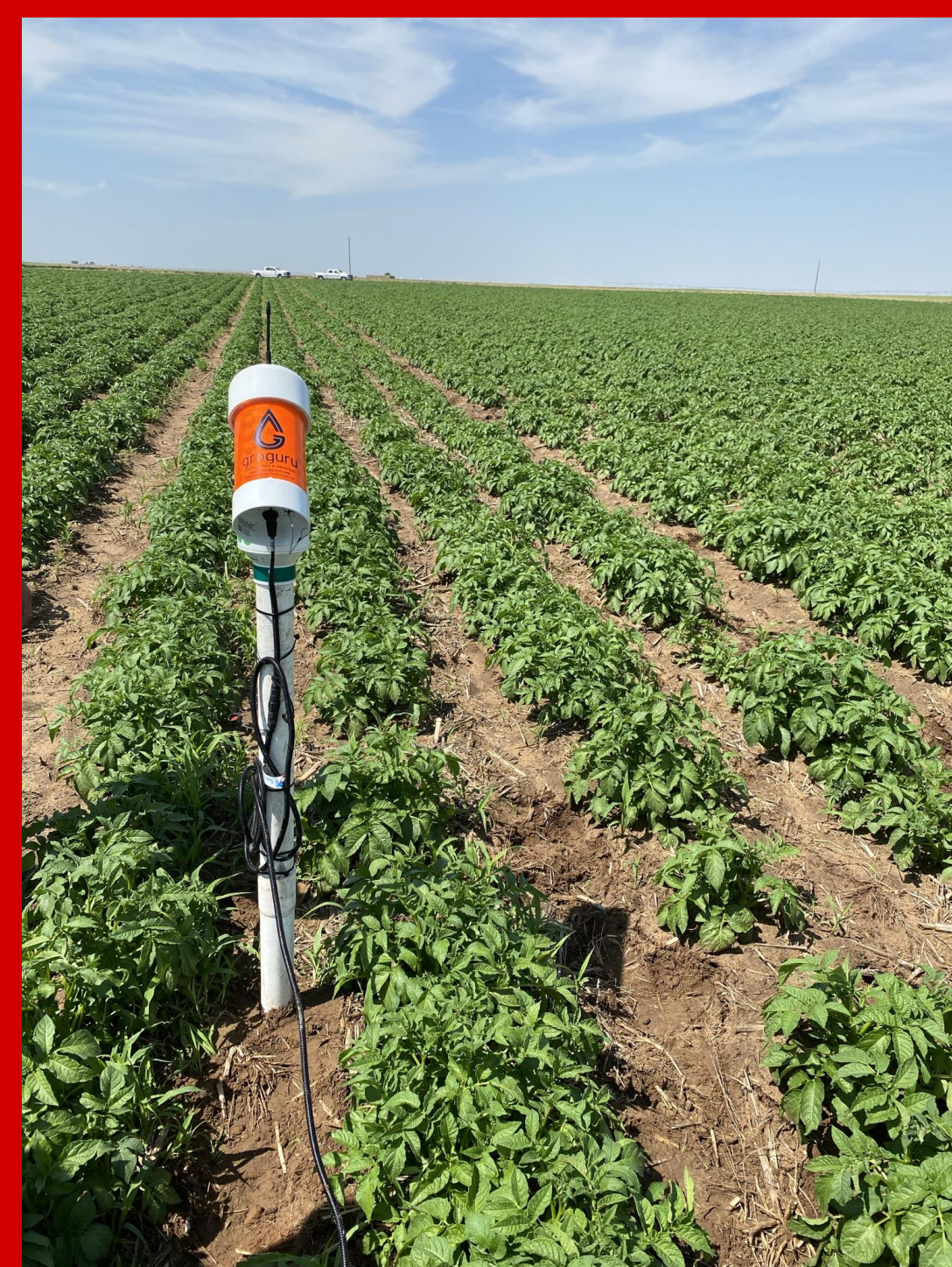
Figure 3. Aboveground telemetry attached to a soil moisture probe (not shown)
